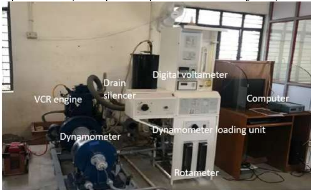
Fig. 5 Photographic view of the experimental setup for a variable compression ratio engine
