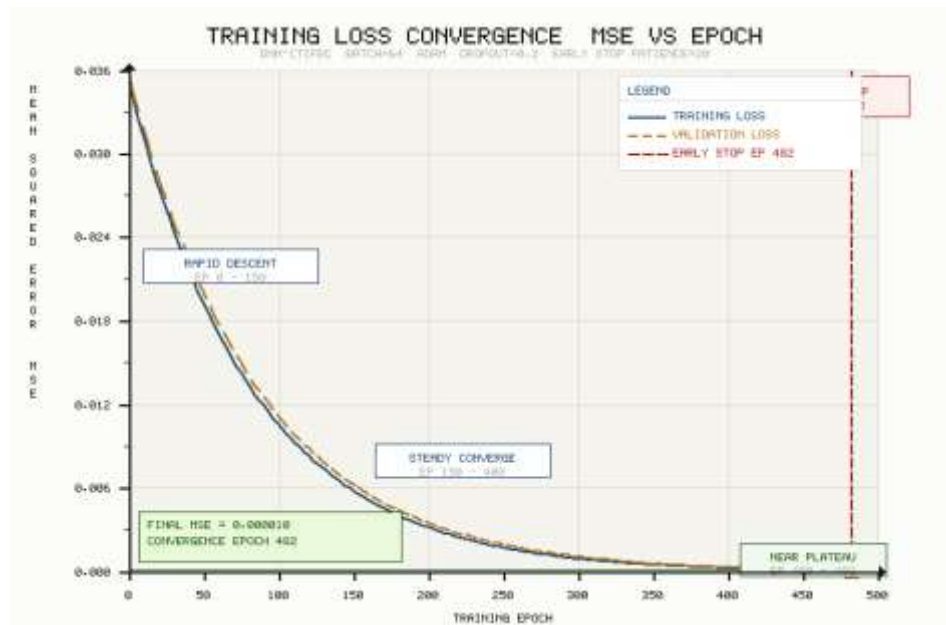
Figure 5. MSE loss convergence. Navy = training loss; orange dashed = validation loss; red = early stopping at epoch 482. Final MSE = 0.000010.
