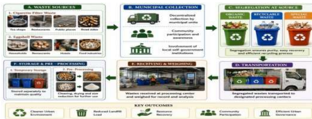
Fig 3.3 Hybrid Biofiller Recovery and Preparation Process
