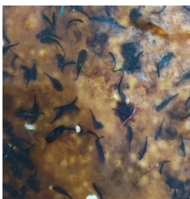
Plate 4.6.15: Half without dye and half Rose dye extract, Tamarind Seed Powder Bio-film.
