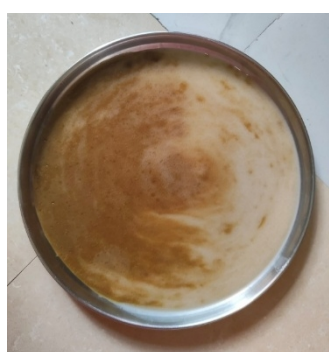
Plate 4.6.6: Half without dye and half Rose dye extract, Tamarind Seed Powder Bio-film.
