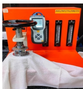
PLATE 6: AIR PERMEABILITY TESTER
