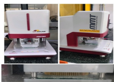
PLATE 5: SDL ATLAS M290 MOISTURE MANAGEMENT TESTER (MMT)
