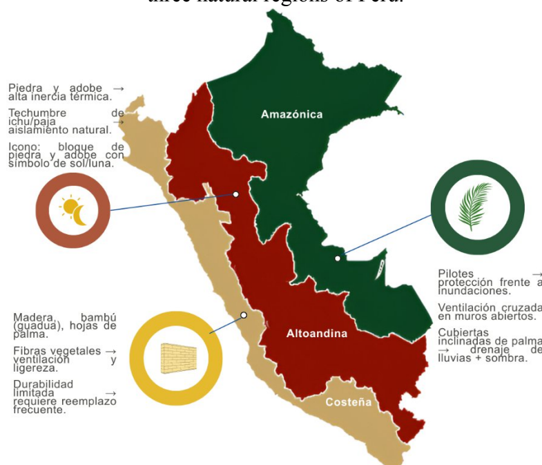
Figure 5. Relationship between local materials and their physical-environmental performance in the three natural regions of Peru.
