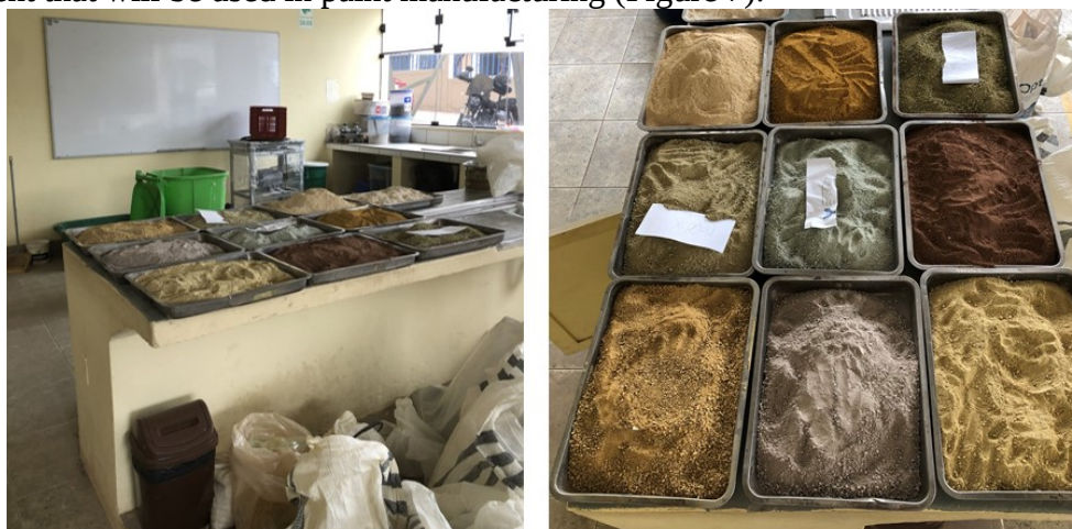
Figure 7. Pigments obtained by sedimentation and bead milling
