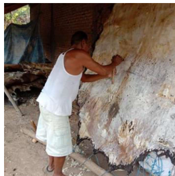
Figure 5. The process of "scraping" buffalo skin
