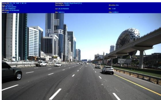
Figure 4: LCMS-2 ROW Image & Photogrammetry Assets Data Collection (RTA, 2024)
